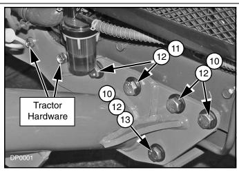
Figure 2. Right Mount Installed
